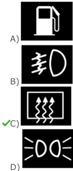
Question 38. In the car's instrument panel, which one of the following warning lights is illuminated indicates that the rear windshield resistance is working?
